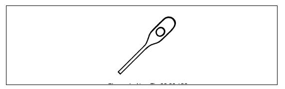
To aid with the removal of pins and sockets from all types of connectors, a new tip has been added to the pin removal tool, P/N 85 80 110 and to spare tip set, P/N 85 80 128.
