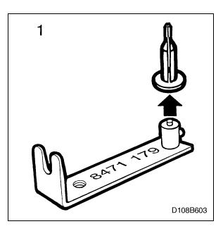
2 Insert the forked part of the tool under the head of the expander rivet and withdraw same.
