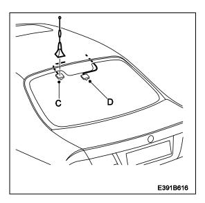
The best location for the antenna is described in installation instructions 47 12 303 included with kit 400 106 712. Cable laying will be simple and the antenna will not be visible in the rear-view mirror.
