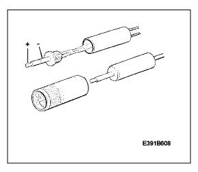
Use an ohmmeter to determine which of the terminals is the (+) and (-) of the jack plug. Solder the brown/grey lead in pos. 10 on the adapter cable to the (+) terminal on the jack plug. Solder the green lead in pos. 3 on the adapter cable to the (-) terminal on the jack plug.
