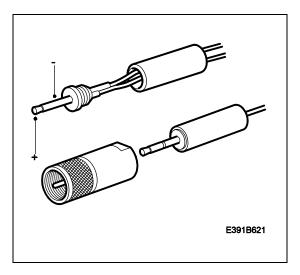
Use an ohmmeter to determine which of the terminals is the (+) and (-) of the jack plug. Solder the brown/grey lead in pos. 10 on the adapter cable to the (+) terminal on the jack plug. Solder the green lead in pos. 3 on the adapter cable to the (-) terminal on the jack plug.
