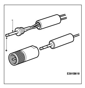
Use an ohmmeter to determine which of the terminals is the (+) and (-) of the jack plug. Solder the brown/grey lead in pos. 10 on the adapter cable to the (+) terminal on the jack plug. Solder the green lead in pos. 3 on the adapter cable to the (-) terminal on the jack plug.
