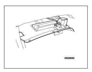
2 Detach the pedal connectors for the brake pedal by turning them 90° clockwise and pulling them out.
