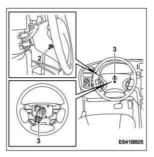
3 Lift out the module and unplug the cable connections.
