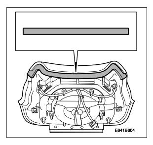
Fit the weatherstrip along the inner edge as illustrated. Press the strip firmly in place.
