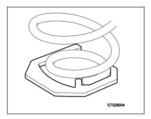
If the gauge does **not** pass over the outer diameter of the bottom spring coil, the spring must be changed, see Service Manual 7:1, "Adjustment/replacement, Springs, page 53.
