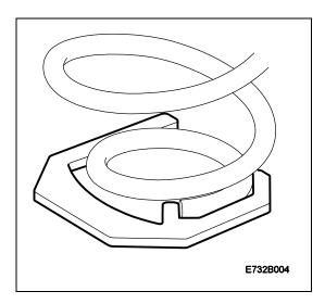
3 Insert the gauge with one shank on each side of the bottom coil of the spring.
