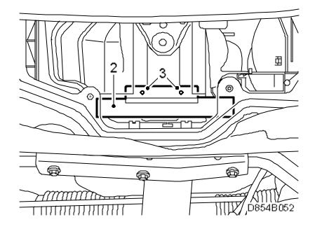
3. Drill a 1.5 mm hole using the air deflector as a template. Drill in the centre of the hole but not deeper than 5 mm as the evaporator may be damaged.
