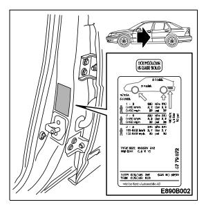
Cars with base solid finishing paint have a label with the text **BODYCOLOUR IS BASE SOLID**. The label is located on the left-hand B-pillar, next to the ordinary colour code and tyre pressure label.
