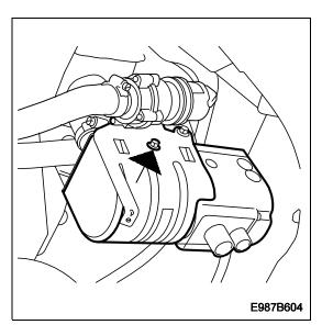
Suspend the holder with heater from the hook at the front of the bracket and screw the heater in place. Tighten the two screws that secure the heater in the holder.
