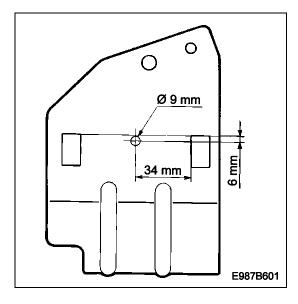
2 File the holes and remove any filings and flakes of paint. Clean with Teroson FL cleaner. Apply Standox 1K Füllprimer. Apply a top coat.
