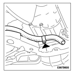
Remove the rubber protection from the clip that holds the exhaust hose of the heater to the subframe. (The clamp in included in the kit and is marked as size 24.)
