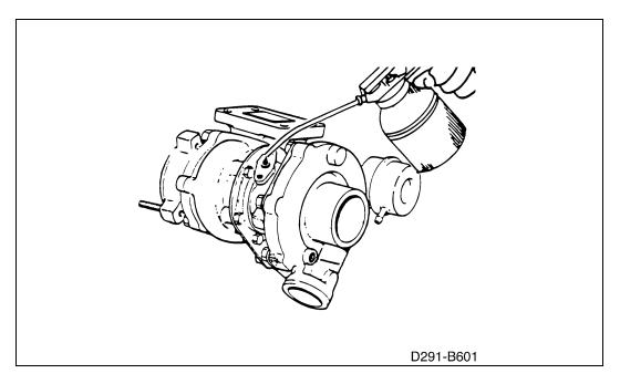
Replacement turbo units can be seriously damaged by inadequate initial lubrication, with the result that they have to be scrapped.
