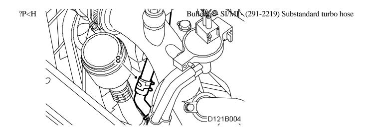
10. Fit the elbow hose to the T-piece.
