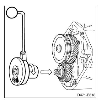
8 Subtract the average reading for the input shaft from the average reading for the output shaft. The calculated tension is a measure of the output shaft turning torque, normally 50-100 N/cm. Example: reading on output shaft = 110 N/cm and reading on input shaft = 30 N/cm gives 110 - 30 = 80 N/cm.
