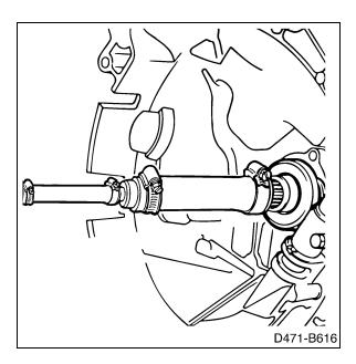
4 Quickly rotate the input shaft back and forth. Measurement can start when the shaft moves freely.
