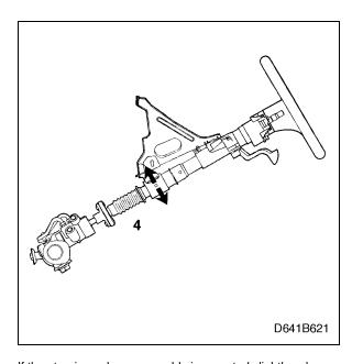
If the steering column assembly is mounted slightly askew, squeaking or creaking sounds may occur when the steering wheel is turned. This is due to clamping forces arising between the steering column assembly and the steering column, which subject the felt bearing (4) to a concentrated load. This can also give rise to stiff steering wheel adjustment or heavy steering.
