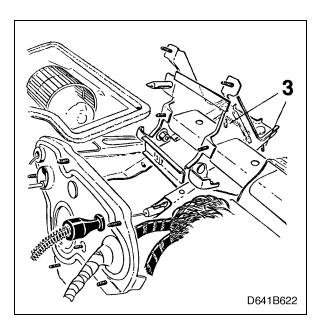
7 First slacken the steering column assembly's upper retaining nuts (2) a few turns and then undo the lower retaining bolt (1). Use a 13 mm hex socket with flexible extension bar to angle the bolts.
