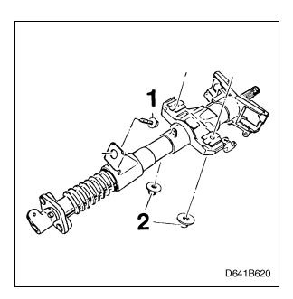
5 Release the steering wheel adjustment lever and pull the steering wheel back and forth a few times. Lock the adjustment lever and tighten the upper retaining nuts (2).
