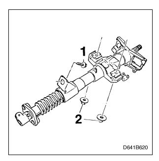
8 Tighten the two upper retaining nuts (2) by hand until the steering column assembly bracket abuts against the steering column "basket".
