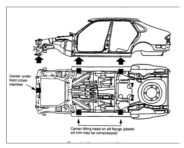
Take care when putting a new style 900 onto a lift or when using a jack to elevate the car. Please see the figure below for the locations for appropriate lifting and jacking points.
