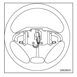
M96 - M97 with horn connector in 6 o'clock position.
