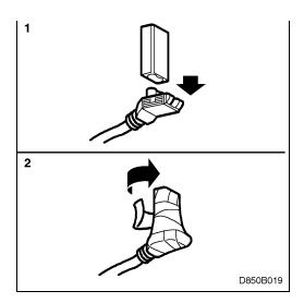
2 Wind at least three turns of tape round the connector and resistor.
