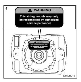
5 Refit the airbag unit in the steering wheel and tighten the screws.
