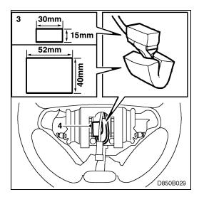
4 Place the connector inside the steering wheel and tuck it down as shown.
