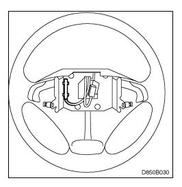
M95 - M96 with horn connector in 9 o'clock position.
