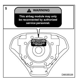
6 Refit the airbag unit in the steering wheel and tighten the screws.
