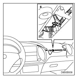
7 Affix label above the switch on the airbag module.
