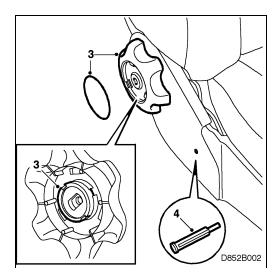
4 Press out the expansion pin in the cover between the seat-back adjusting mechanism and the seat frame, and carefully remove the cover.
