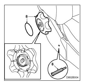
9 Continue on the other side of the seat. Undo the screw and remove the sleeve, using pliers if the sleeve proves stubborn.
