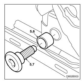
6 Fit the new sleeve and check that it turns freely. If not, use a file to smooth the shank.
