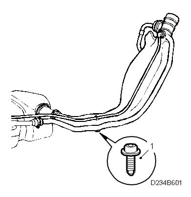
The hose on the EVAP canister on a small number of cars may have been bent due to incorrect assembly on the production line. This can block the system and cause a number of faults that can not primarily be traced to this cause, e.g.
