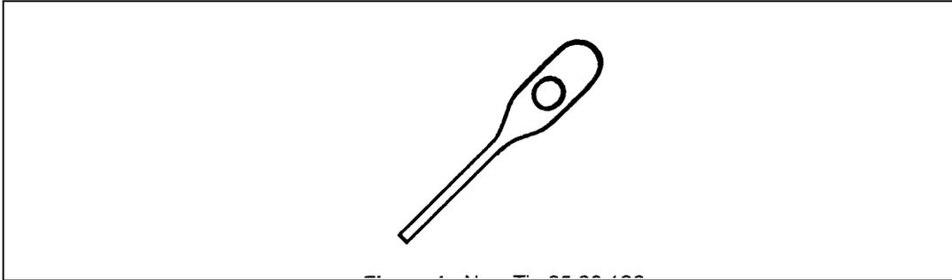
To aid with the removal of pins and sockets from all types of connectors, a new tip has been added to the pin removal tool, P/N 85 80 110 and to spare tip set, P/N 85 80 128.
