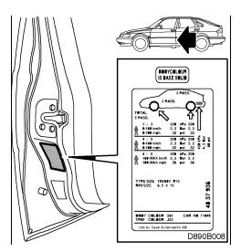
Cars with base solid finishing paint have a label with the text BODYCOLOUR IS BASE SOLID. The label is located on the lower part of the left-hand front door, next to the ordinary colour code and tyre pressure label.
