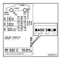
When all production cars are painted with base solid finishing paint, the label will be discontinued. Instead, the ordinary colour code and tyre pressure label will have the text BASE SOLID.
