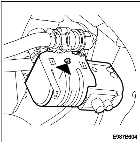
Suspend the holder with heater from the hook at the front of the bracket and screw the heater in place. Tighten the two screws that secure the heater in the holder.
