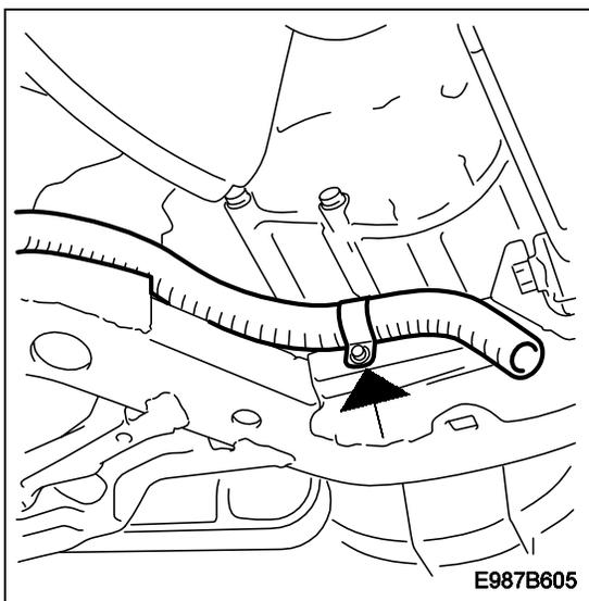
Remove the rubber protection from the clip that holds the exhaust hose of the heater to the subframe. (The clamp is included in the kit and is marked as size 24.)
